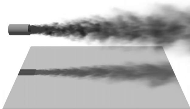
Fig. 23. Volumetric rendering of the mixture fraction of helium for the variable density jet.
